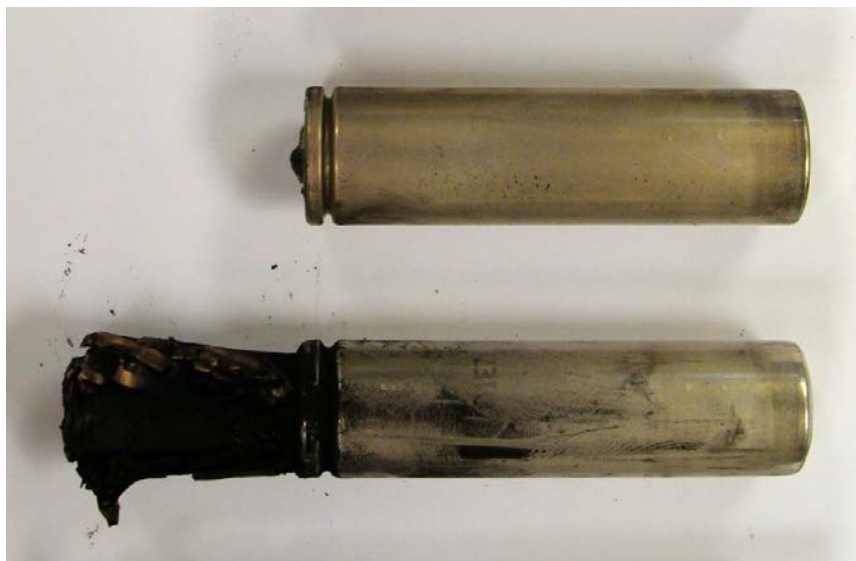
Figure 8. LIBs after thermal runaway in the bomb calorimeter: the top cell did not eject its contents, but the bottom cell did
