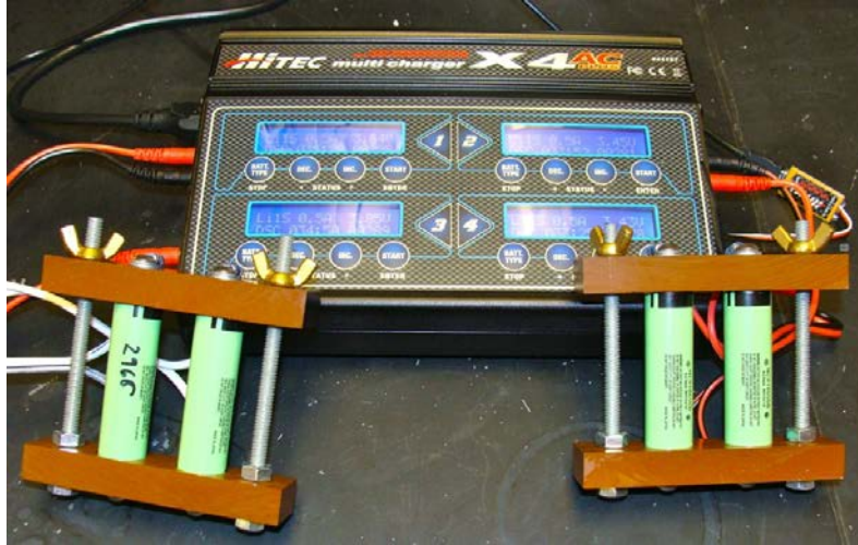
Figure 2. Battery charger and fixtures used to charge four cells individually and simultaneously
